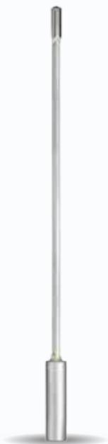
ACCUSHARP Gun drills are straight fluted drills which allow cutting fluid (either compressed air or a suitable liquid) to be injected through the drill's hollow body to the cutting face. ACCUSHARP drills used for deep drilling—a depth-to-diameter ratio of 300:1 or more is possible.
